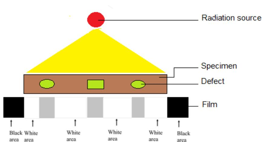
**Figure 1.** Schematic of radiography set-up
