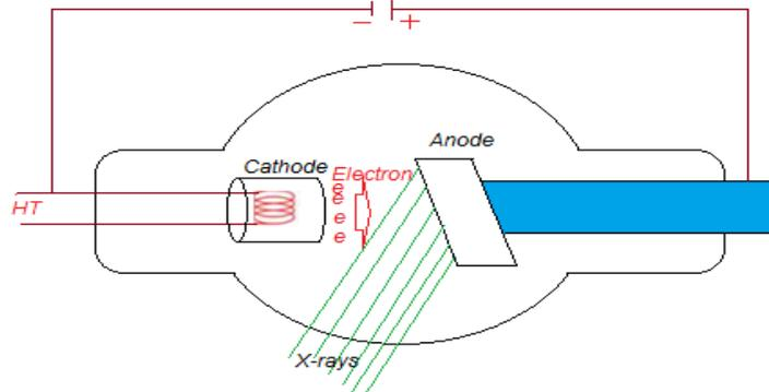
**Figure 2.** Basic x-ray production process
