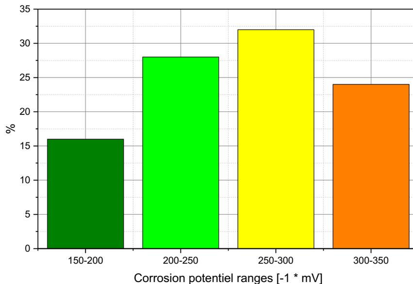
**Figure 4.** relative frequency of corrosion potentials
