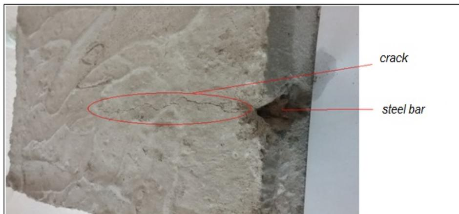
**Figure 5.** Specimen n°3 which presents a crack
